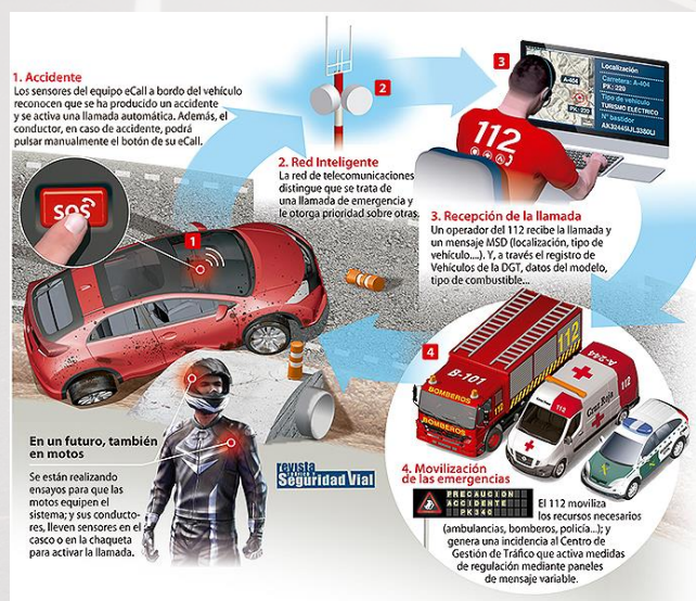
Illustration 115. how eCall works in Spain. Source: DGT Magazine
