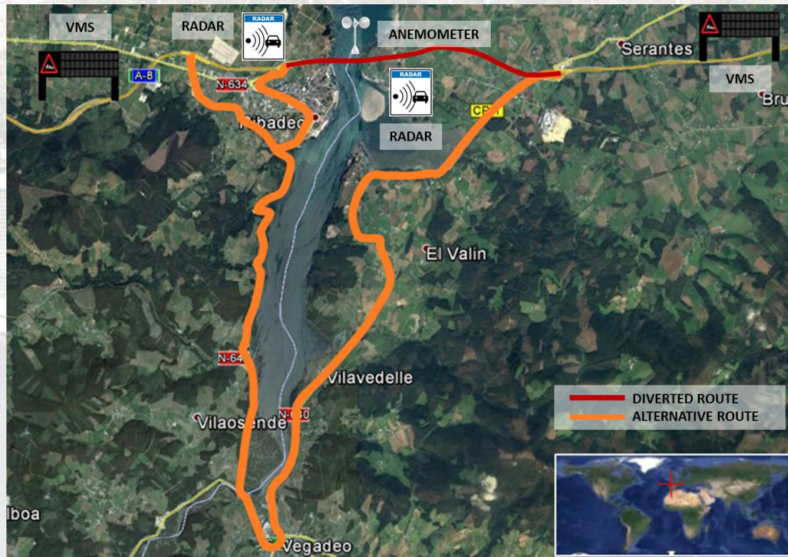
Illustration 46. Automated detour scheme for the Puente de los Santos. Source: DGT
