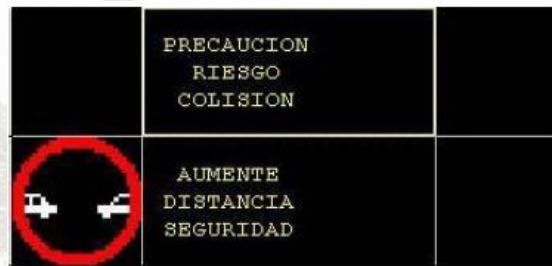
Illustration 56. Signalling alternation in case of safety distance not being met. Source: DGT
