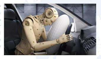
Strapped into car seats and propelled at speed, they are designed to measure the effect and the impact of real-life crash situations and highlight potential injury. For car buyers, these tests give invaluable information about just how safe a car is for both driver and passengers as safety ratings are awarded by the European New Car Assessment Programme (EuroNCAP) to all new cars.
