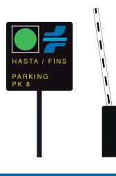
The automatic road barrier will lift upon recognizing the license plate of an authorized vehicle. If plate recognition fails, authorized users can scan a **QR code** at the reader located next to the intercom to open the barrier.
